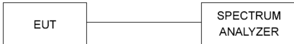
Figure 6 – Peak Output Power Measurements Test Setup
