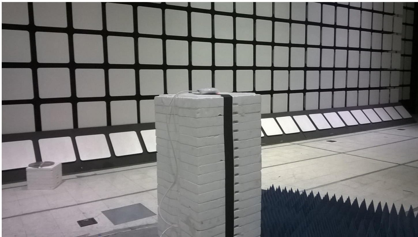
Figure 2 - Radiated Emissions Test Setup, 1 – 25 GHz
