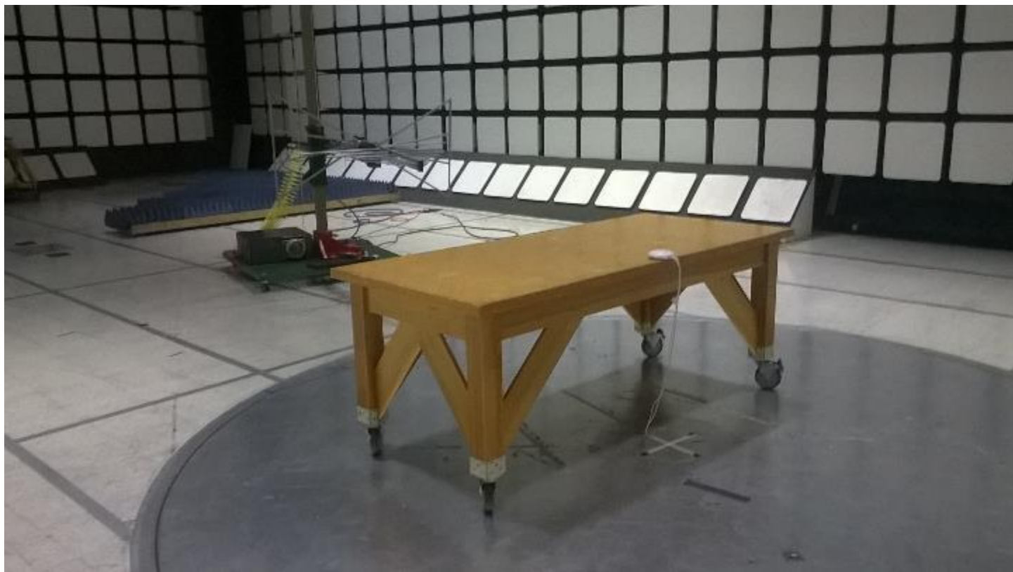
Figure 1 - Radiated Emissions Test Setup, 30MHz - 1GHz
