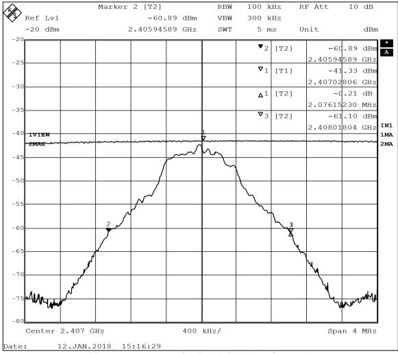
Figure 7 - 99% Occupied Bandwidth, Low Channel.
