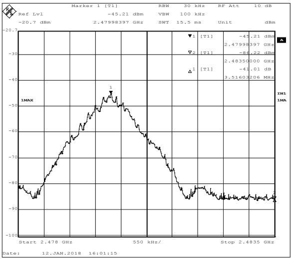
Figure 17 - Band-edge Measurement, High Channel, Fundamental The plot shows an uncorrected measurement, used for relative measurements only. Delta = 41.01 dB; Minimum = 20 dB
