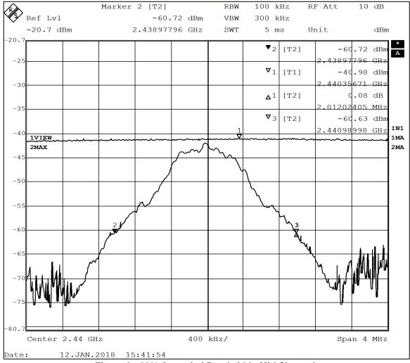
Figure 8 - 99% Occupied Bandwidth, Mid Channel
