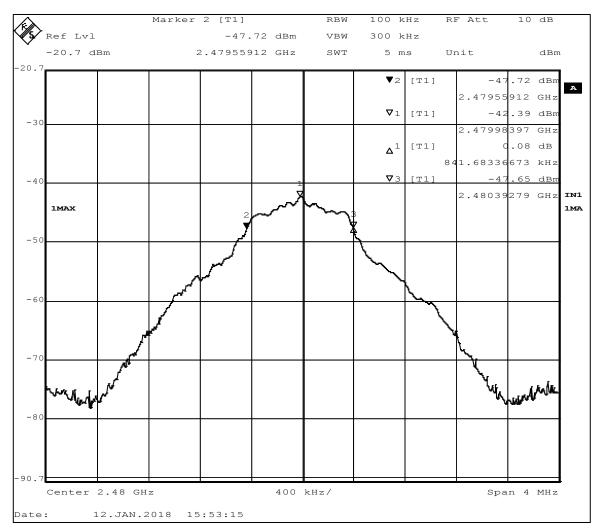
Figure 12 - 6dB Bandwidth, High Channel
