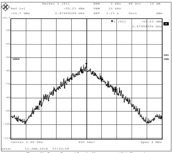
Figure 20 - Power Spectral Density Measurement, High Channel
