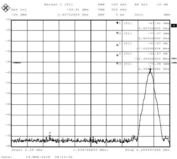
Figure 15 - Unestricted Band-edge Measurement, Low Channel, Fundamental
