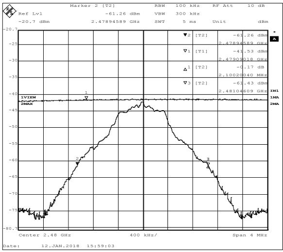
Figure 9 - 99% Occupied Bandwidth, High Channel
