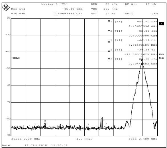
Figure 14 – Restricted Band-edge Measurement, Low Channel, Fundamental The plot shows an uncorrected measurement, used for relative measurements only.
