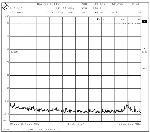
Figure 16 – Restricted Band-edge Measurement, High Channel, Restricted Frequency The plot shows an uncorrected measurement, used for relative measurements only.
