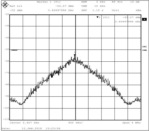
Figure 18 - Power Spectral Density Measurement, Low Channel
