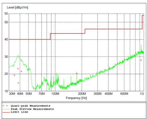
Figure 5 - Radiated Emissions Plot, High Channel
