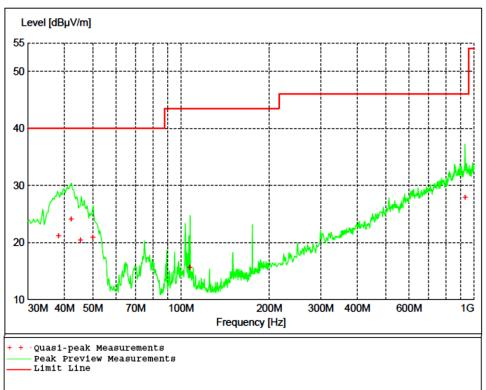
Figure 2 - Radiated Emissions Plot, Receive
