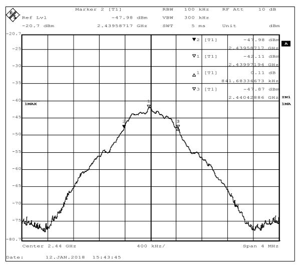
Figure 11 - 6dB Bandwidth, Middle Channel
