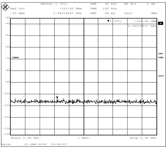
Figure 13 - Band-edge Measurement, Low Channel, Restricted Frequency The plot shows an uncorrected measurement, used for relative measurements only.
