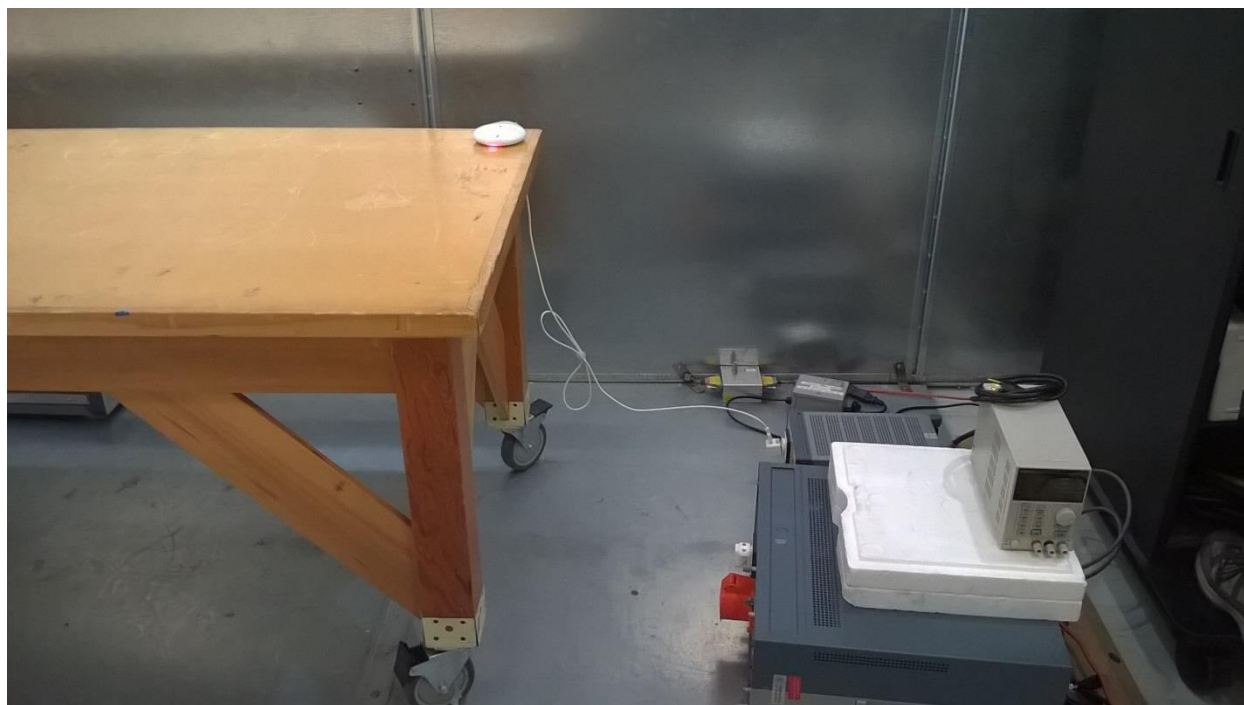
Figure 8 - Conducted AC emissions Test Setup, 150kHz - 30MHz
