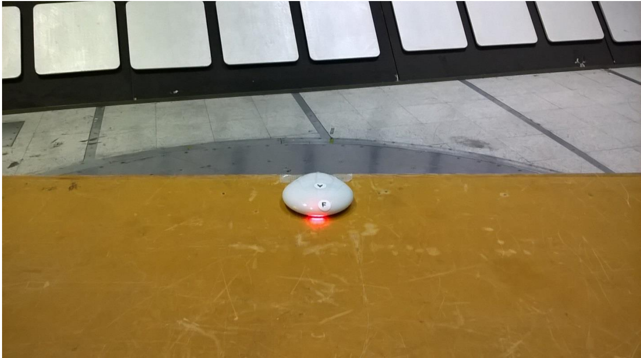
Figure 1 - EUT Test Setup, 30MHz – 1GHz
