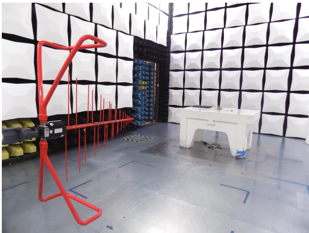
Figure 7 – Radiated Emissions 30 – 1000 MHz, Front View
