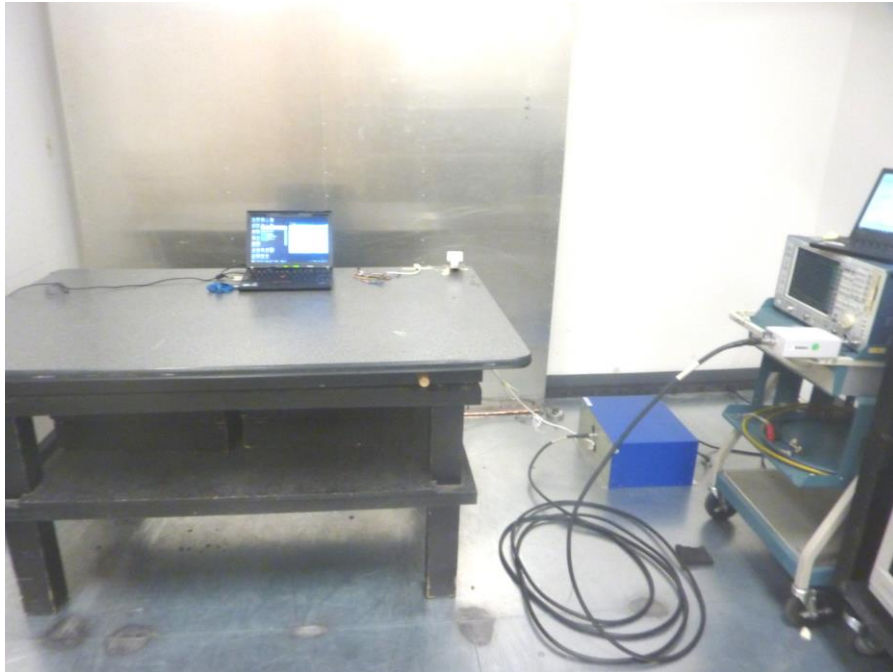
Figure 12 –Conducted Emissions Test Setup
