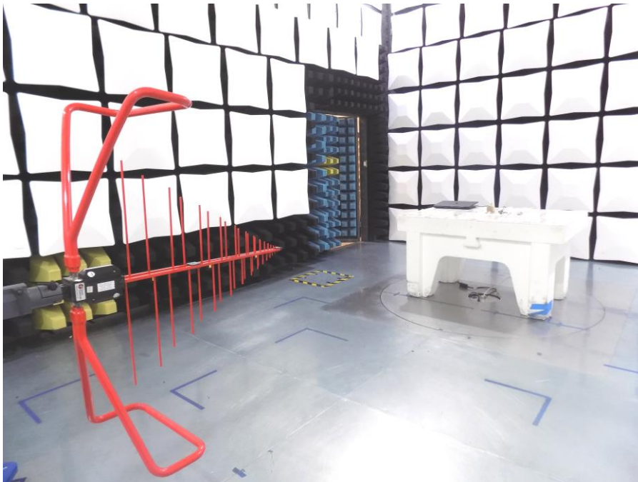
Figure 7 – Radiated Emissions 30 – 1000 MHz, Front View
