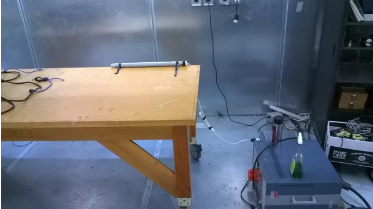
Figure 5 - Conducted emissions test setup
