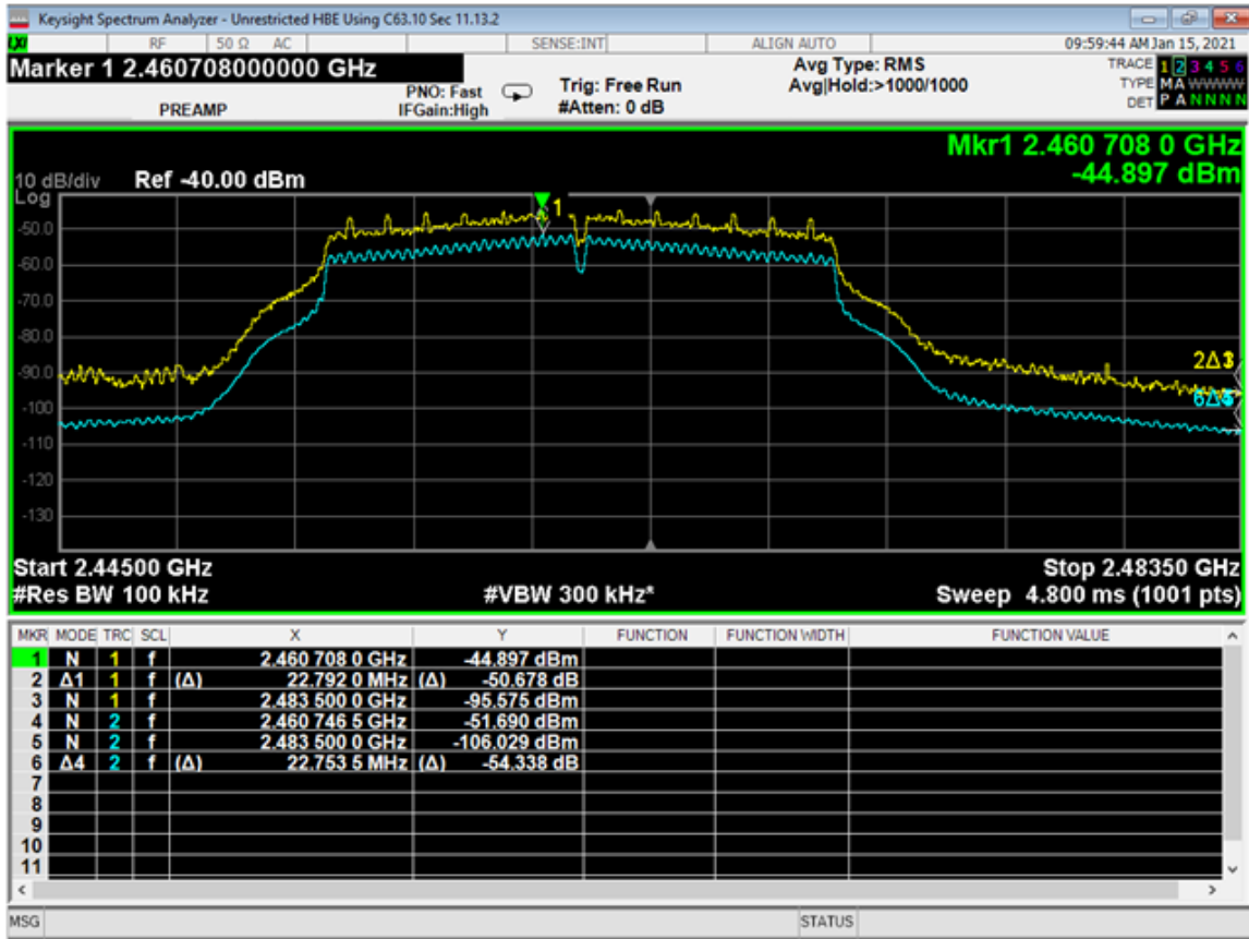
6. 802.11 G Modulation, Higher Band edge, Unrestricted Relative measurements only. Peak measurements are reported in the results table in section 4.0.
