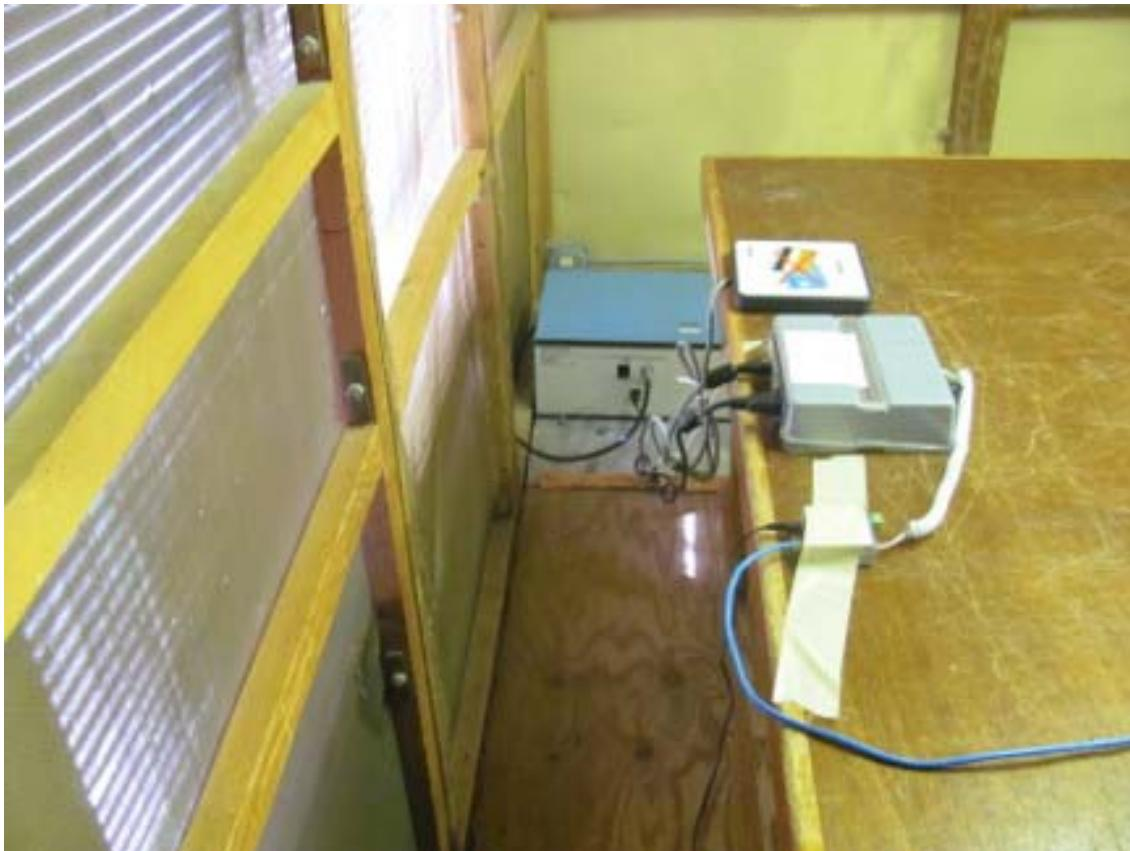
**REAR VIEW****AMERICAN SECURITY SPOL. S R.O.****58 kHz DEACTIVATOR****Model: UXT-P-ADSC****FCC 15.207 and FCC SUBPART B – CONDUCTED EMISSIONS****PHOTOGRAPH SHOWING THE EUT CONFIGURATION
