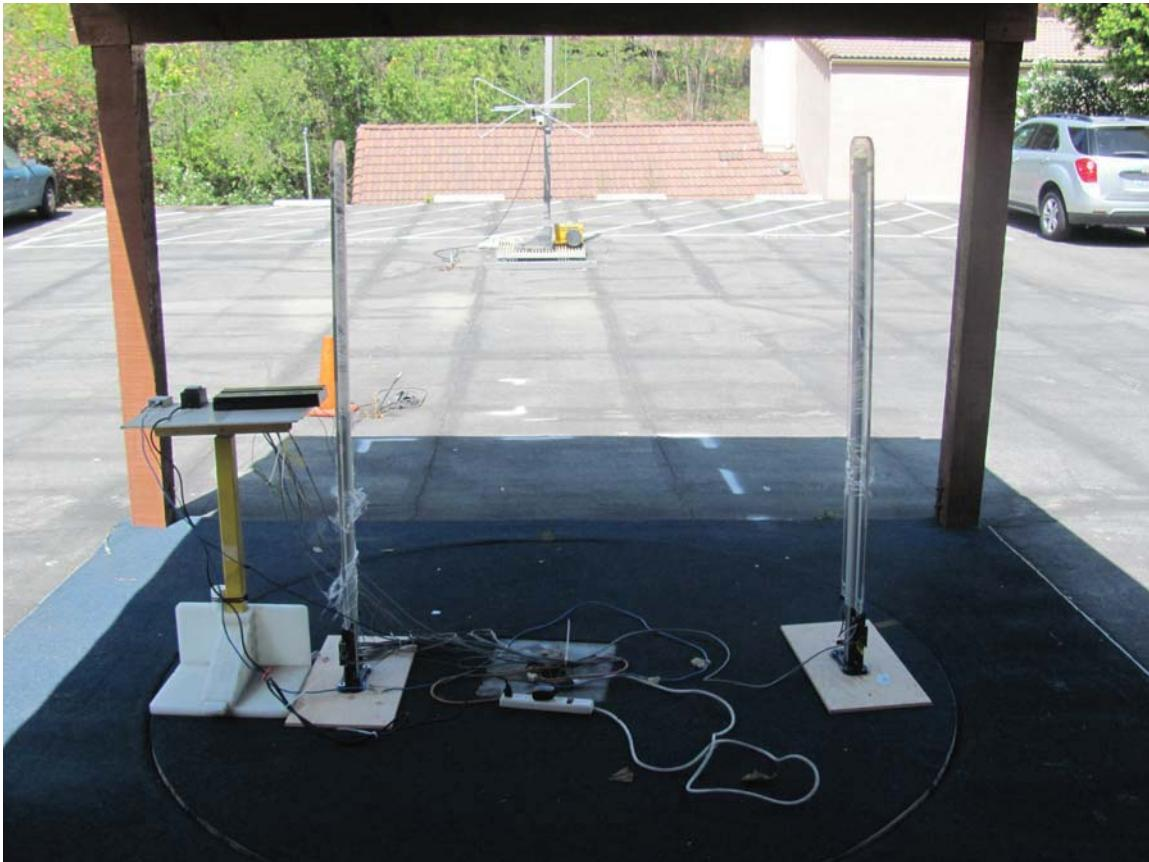
**FRONT VIEW****AMERICAN SECURITY SPOL. S R.O.****20 kHz MMS System****Model: UXT-MMS-NCU****FCC SUBPART B – RADIATED EMISSIONS – ABOVE 30 MHz – SYNC MODE****PHOTOGRAPH SHOWING THE EUT CONFIGURATION
