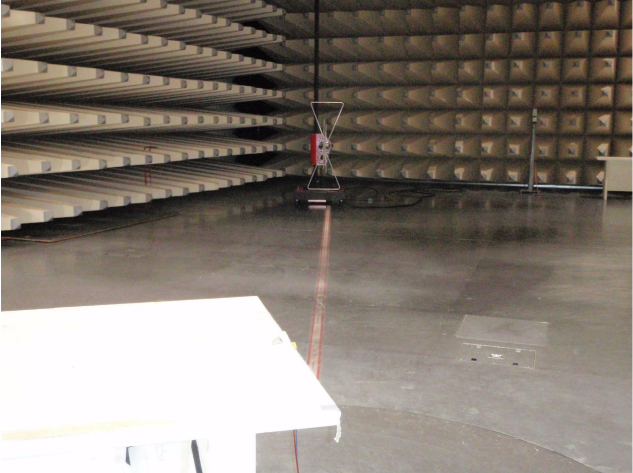
Spurious emission measurement 30 MHz – 1 GHz
