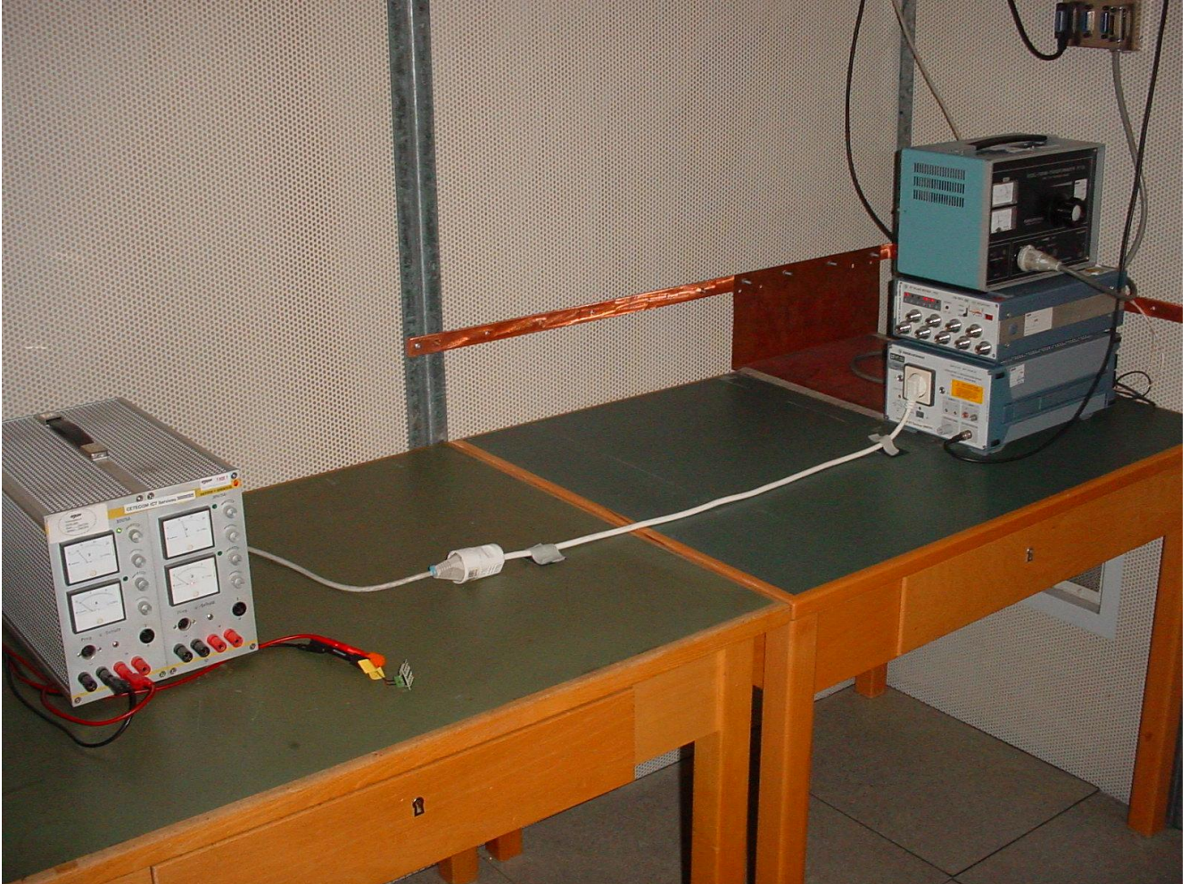
AC conducted line measurement
