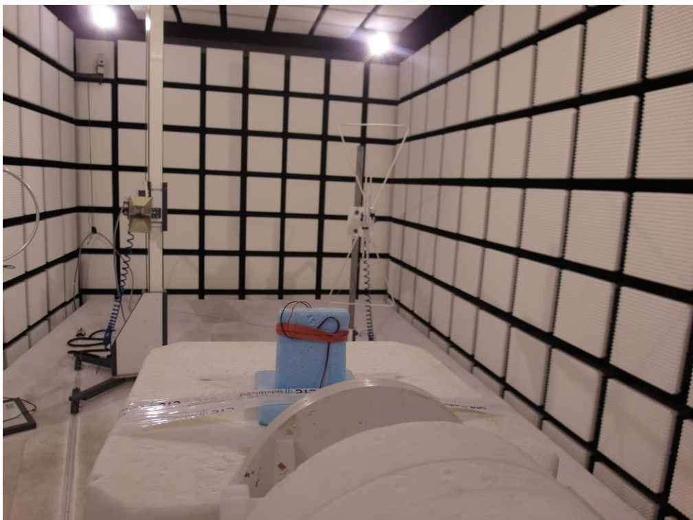
Photo 4: RSE set-up 1 GHz to 18 GHz
