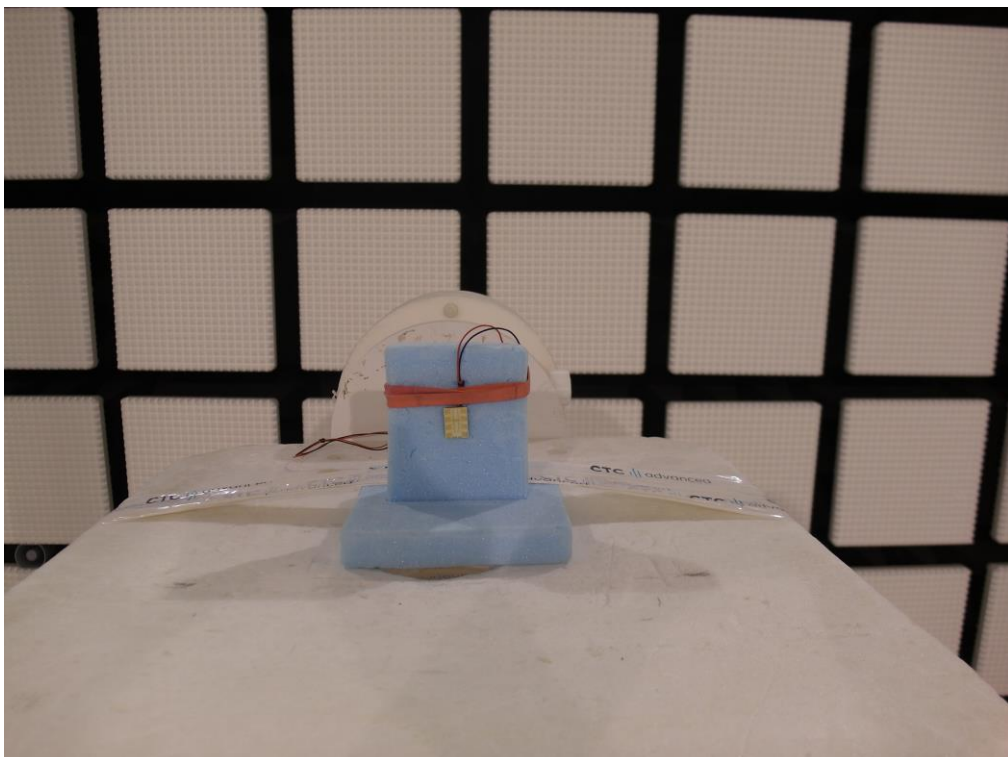
Photo 2: RSE set-up 1 GHz to 18 GHz
