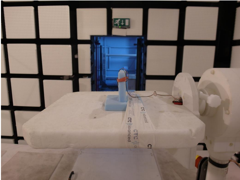
Photo 3: RSE set-up 1 GHz to 18 GHz
