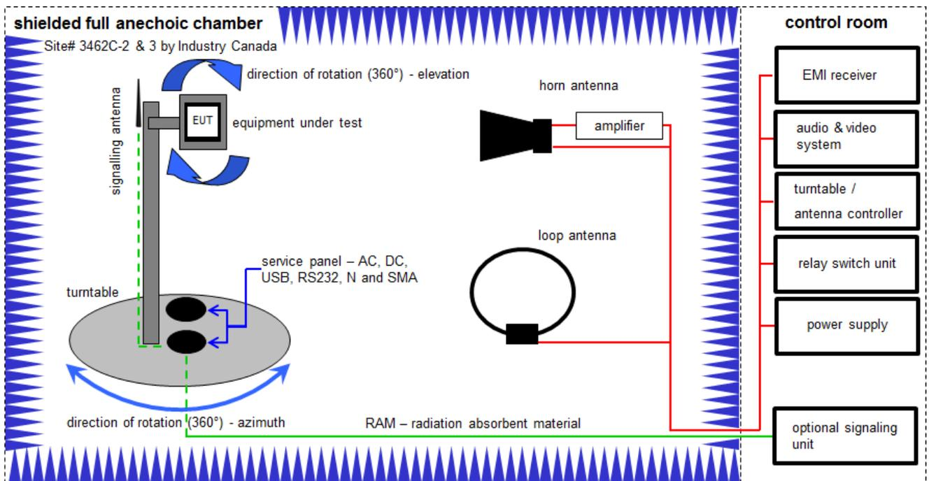
Measurement distance: horn antenna 3 meter / 1 meter; loop antenna 3 meter / 1 meter
