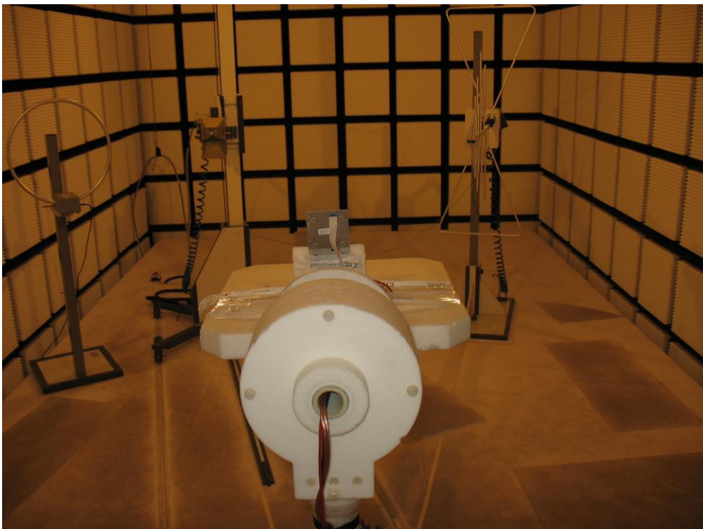
Photo 6: RSE set-up 1 GHz to 18 GHz
