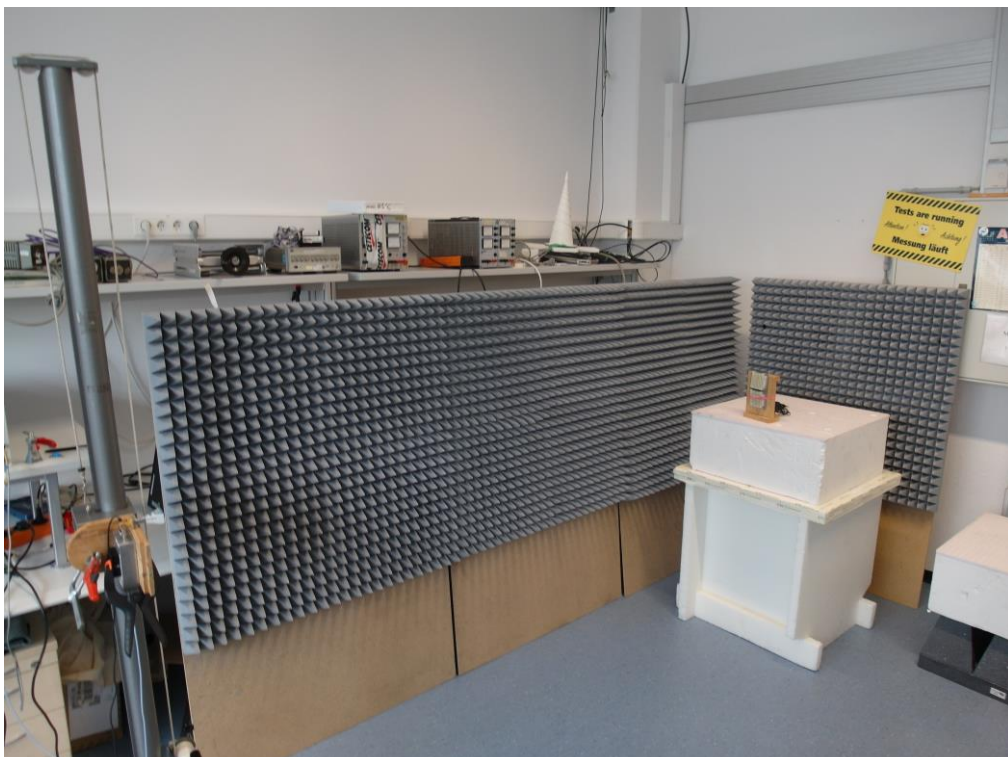
Photo 8: RSE set-up 18 GHz to 110 GHz
