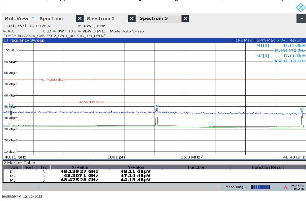
Plot No. 24: 48 GHz, Stopped Mode Low-Middle-High Channel @ AVG detector, horizontal/vertical polarization
