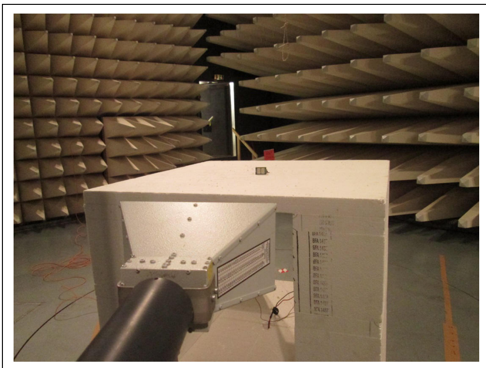
Photograph A1-8: Radiated emissions 6 – 18 GHz at 1 m distance
