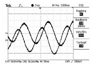
Signal Q is leading if an object moves towards the radar transceiver.
