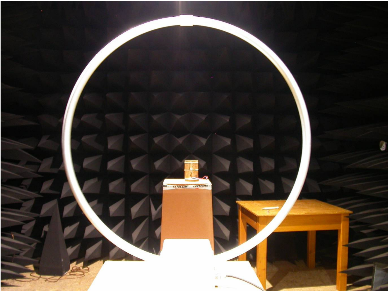
Spurious emission measurement 9 kHz – 30 MHz
