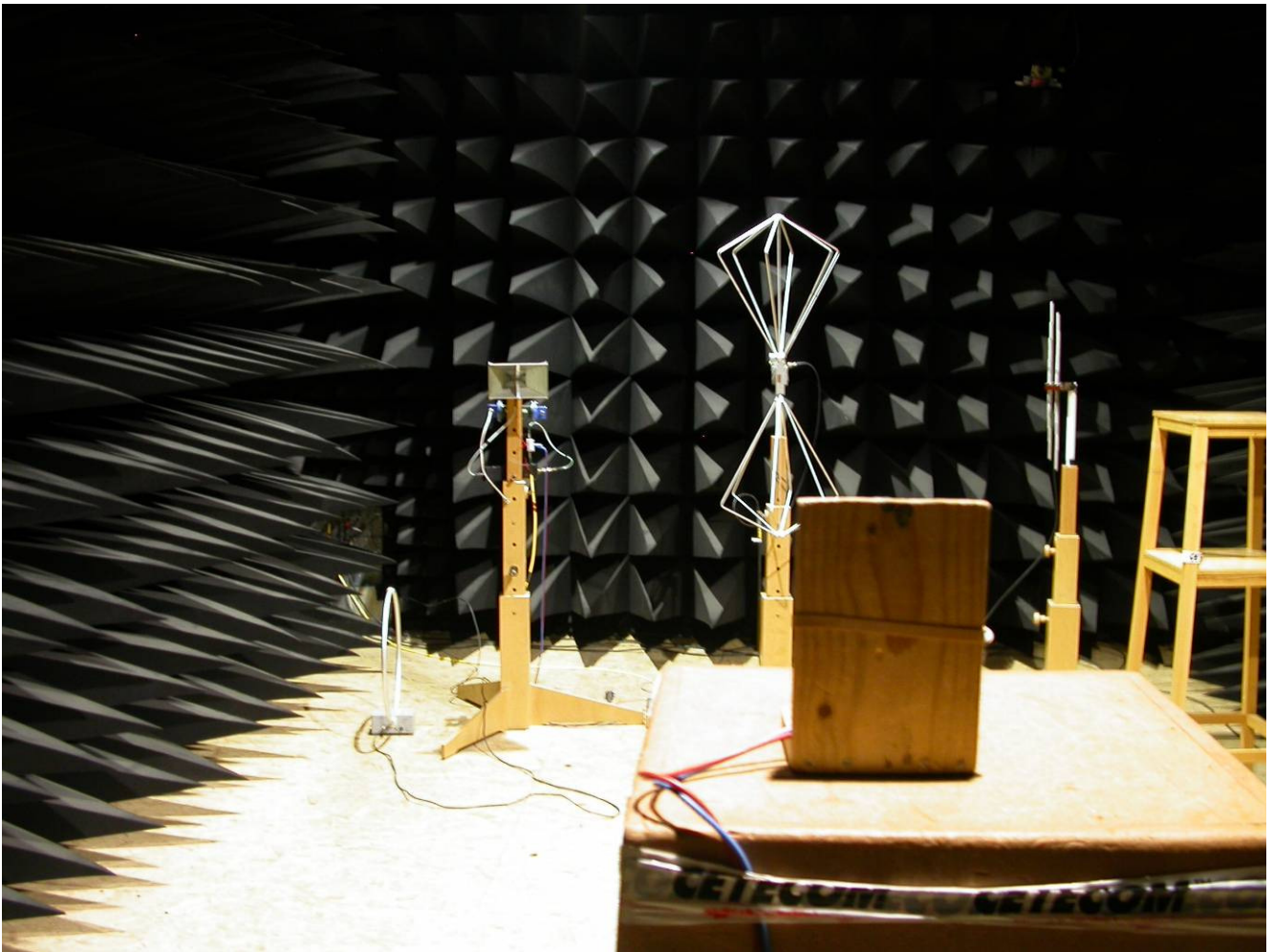
Spurious emission measurement 1 GHz – 12 GHz
