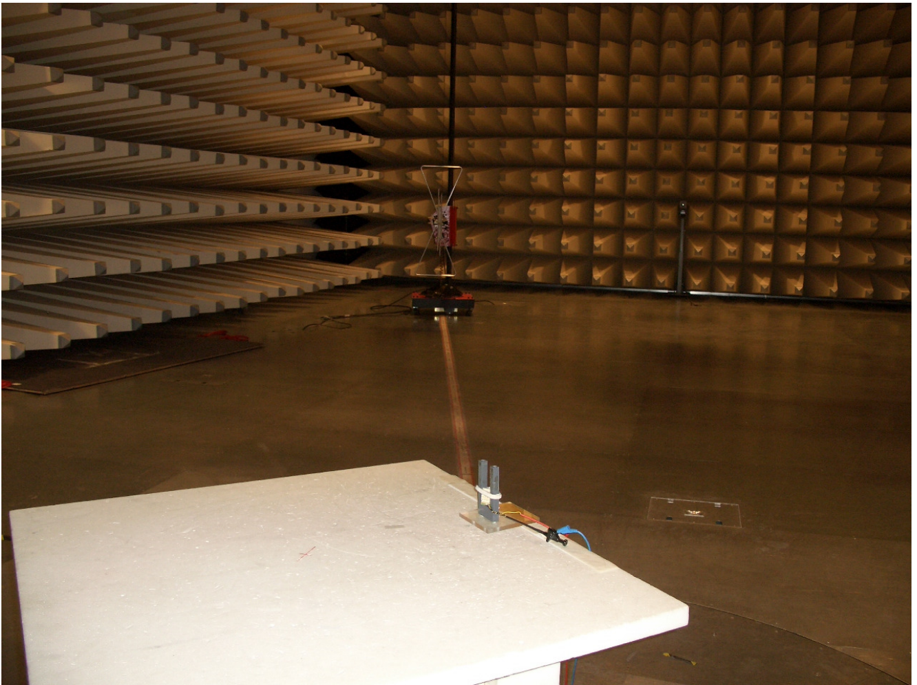
Spurious emission measurement 30 MHz – 1 GHz
