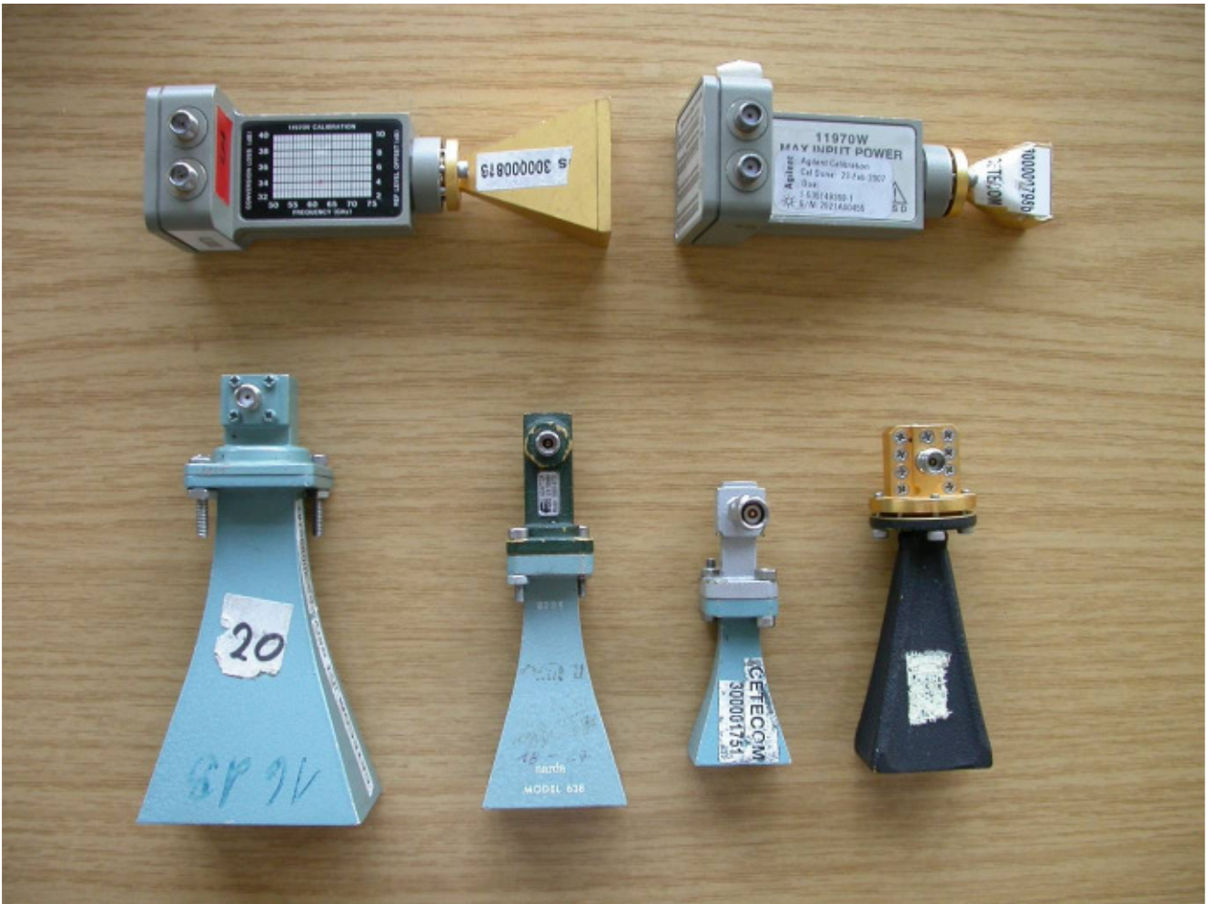
Spurious emission measurement equipment 12 GHz – 110 GHz
