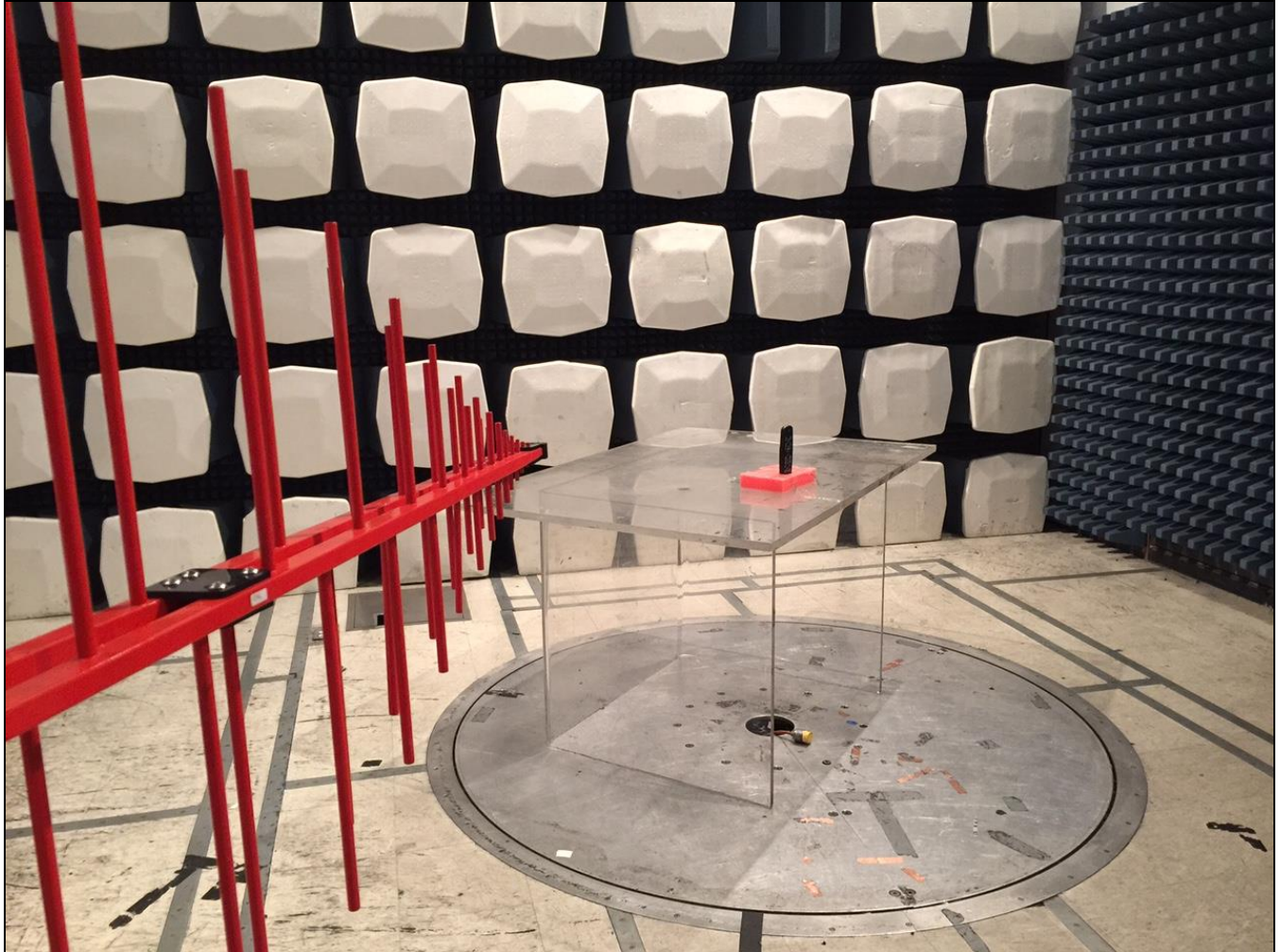
Photograph 1. Field Strength of Fundamental and Harmonics, Test Setup
