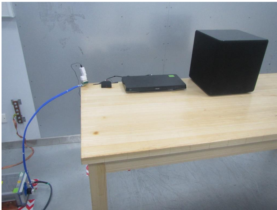
POWERLINE CONDUCTED EMISSIONS MEASUREMENT SETUP
