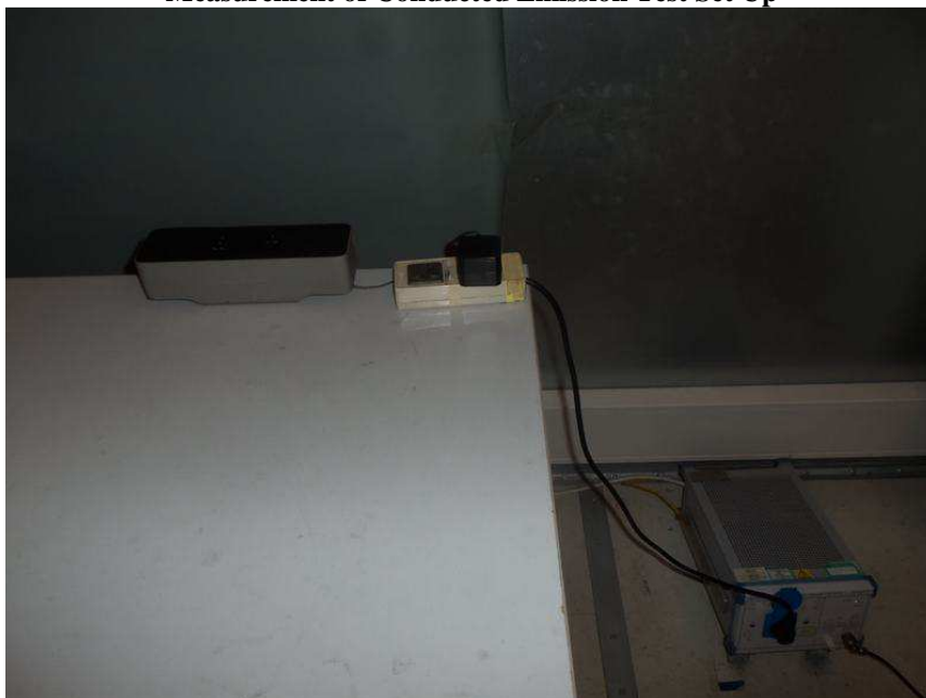
Measurement of Conducted Emission Test Set Up
