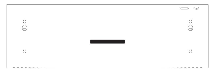
Recess for serial label: Laser etch/CNC: 0.15 Depth
