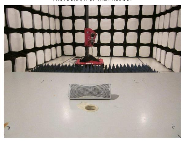
MEASUREMENT OF CONDUCTED EMISSION TEST SET UP
