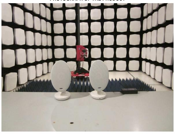
**MEASUREMENT OF CONDUCTED EMISSION TEST SET UP**
