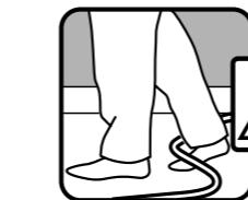
(GB) SAFETY NOTICE! trailing cables are dangerous, secure all cables.
