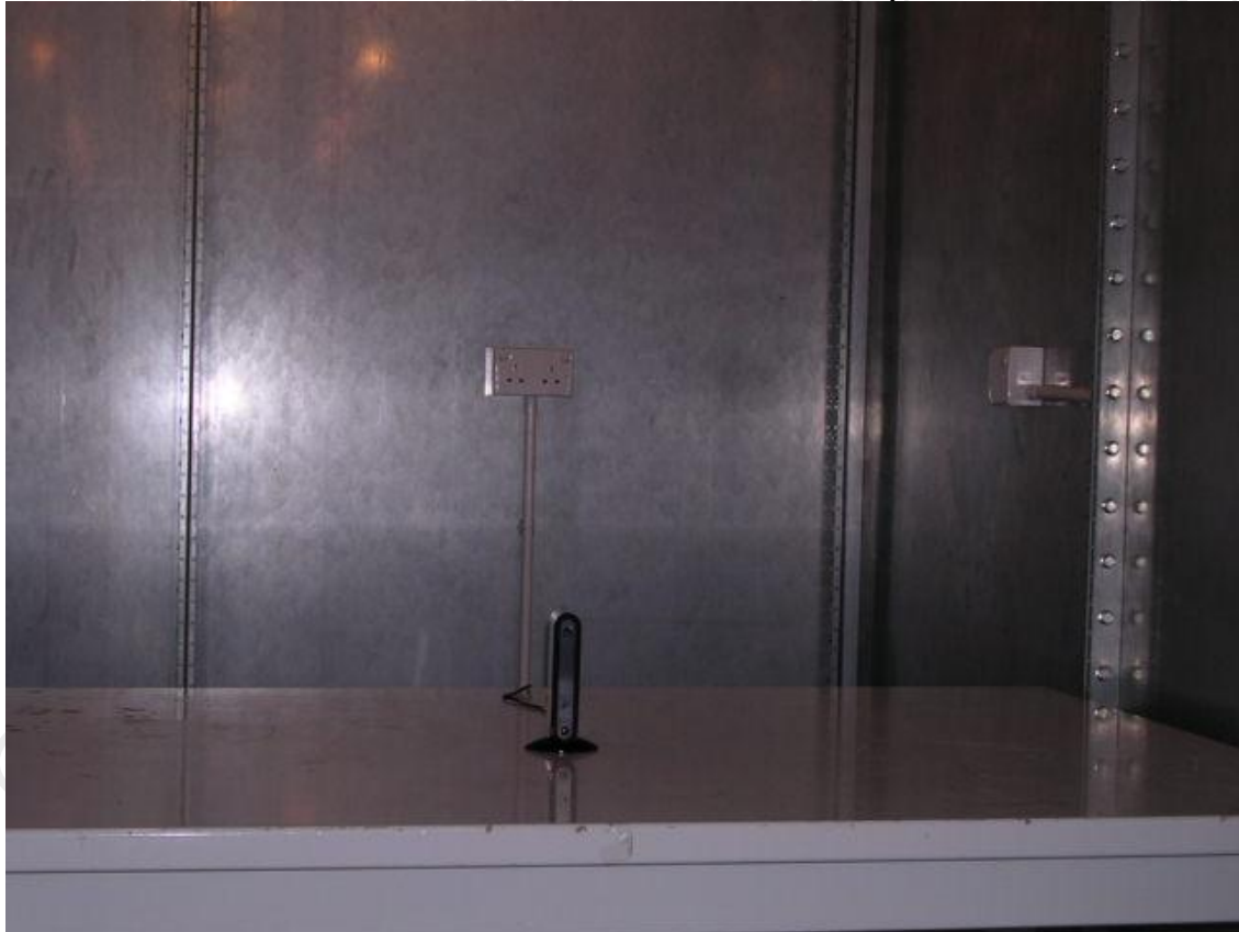
Measurement of Conducted Emission Test Set Up
