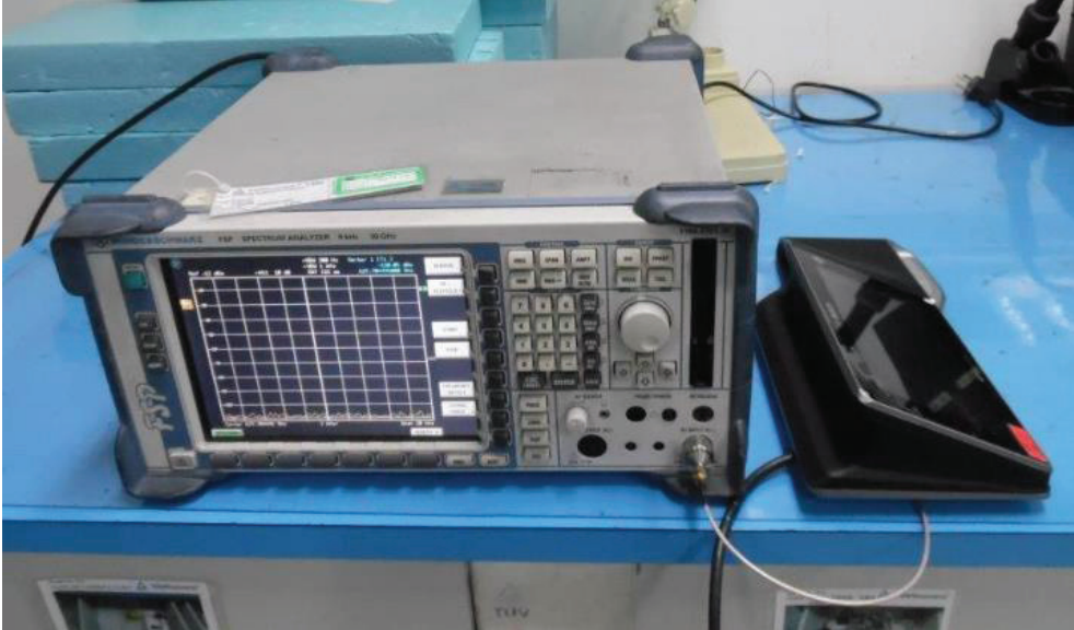
Photograph 2: Set-up for Conducted testing
