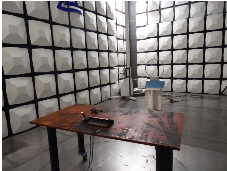
Photograph 1: Set-up for Spurious Emissions (Below 1GHz)
