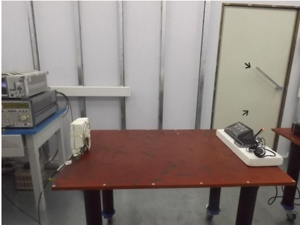
Photograph 4: Set-up for Conducted Emission testing
