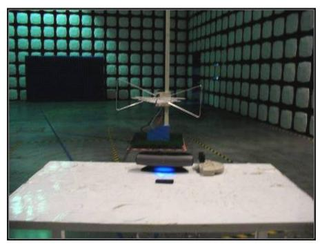
Above 1GHz:(full anechoic chamber)
