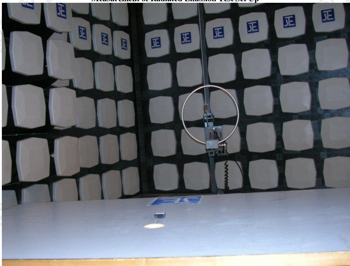
Measurement of Radiated Emission Test Set Up
