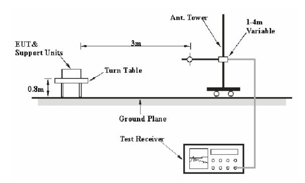
The radiated emission tests were performed in the chamber B test site, using the setup accordance with the ANSI C63.4-2003. The specification used was the FCC 15.209 and 15.235 limits.
