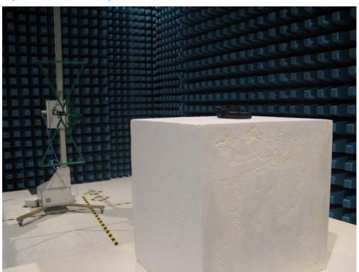
Test Mode: Mode 2: GPRS 1900 Description: EIRP Test Setup
