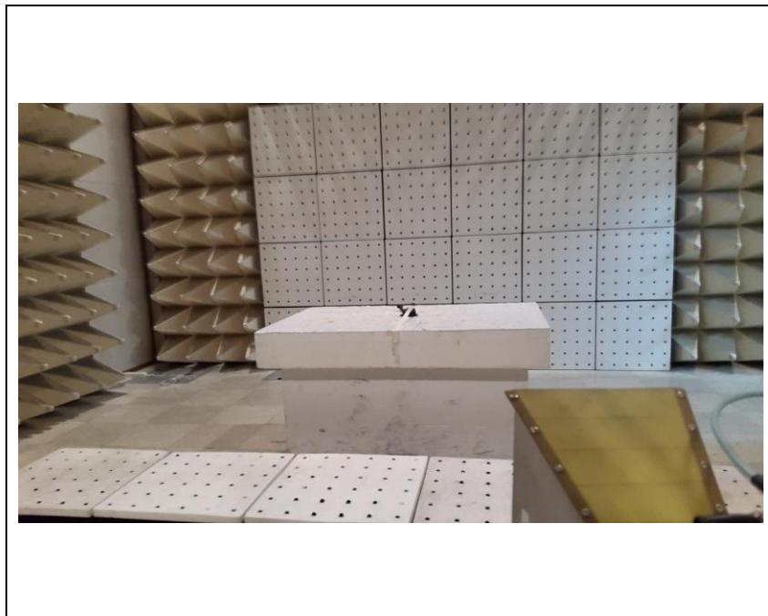
**- DUT was tested in the Z-axis**
