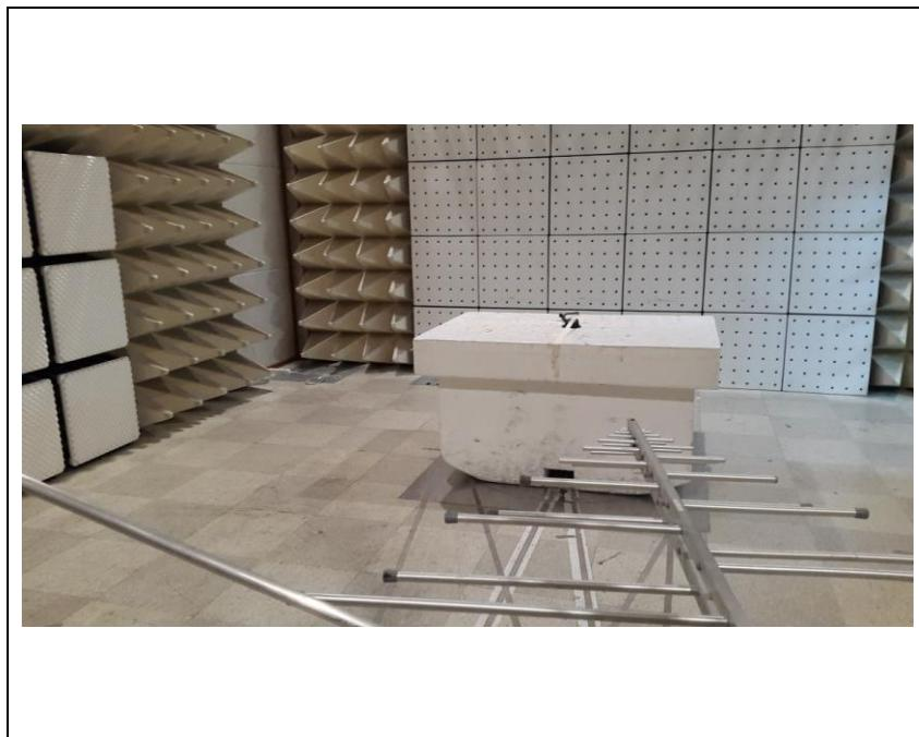
**D. Photo of Test setup (above1 GHz)**
