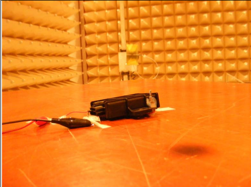
Photo of Field Strength & Spurious Emission Test
