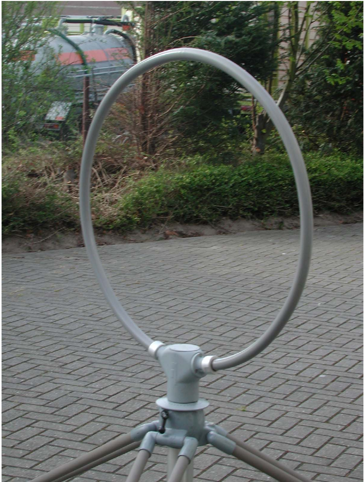
Photograph 3: Test setup radiated emissions <30 MHz (antenna)
