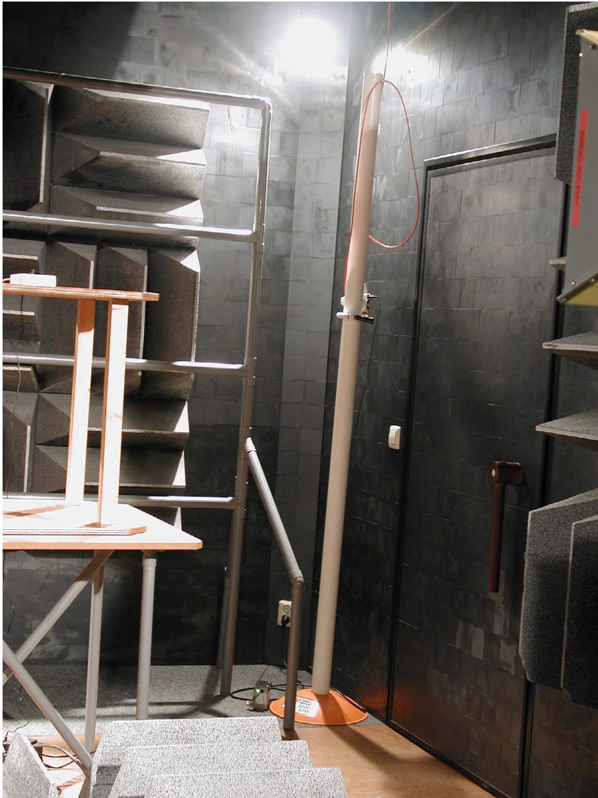
Photograph 11: Test setup radiated emissions > 1 GHz (server)
