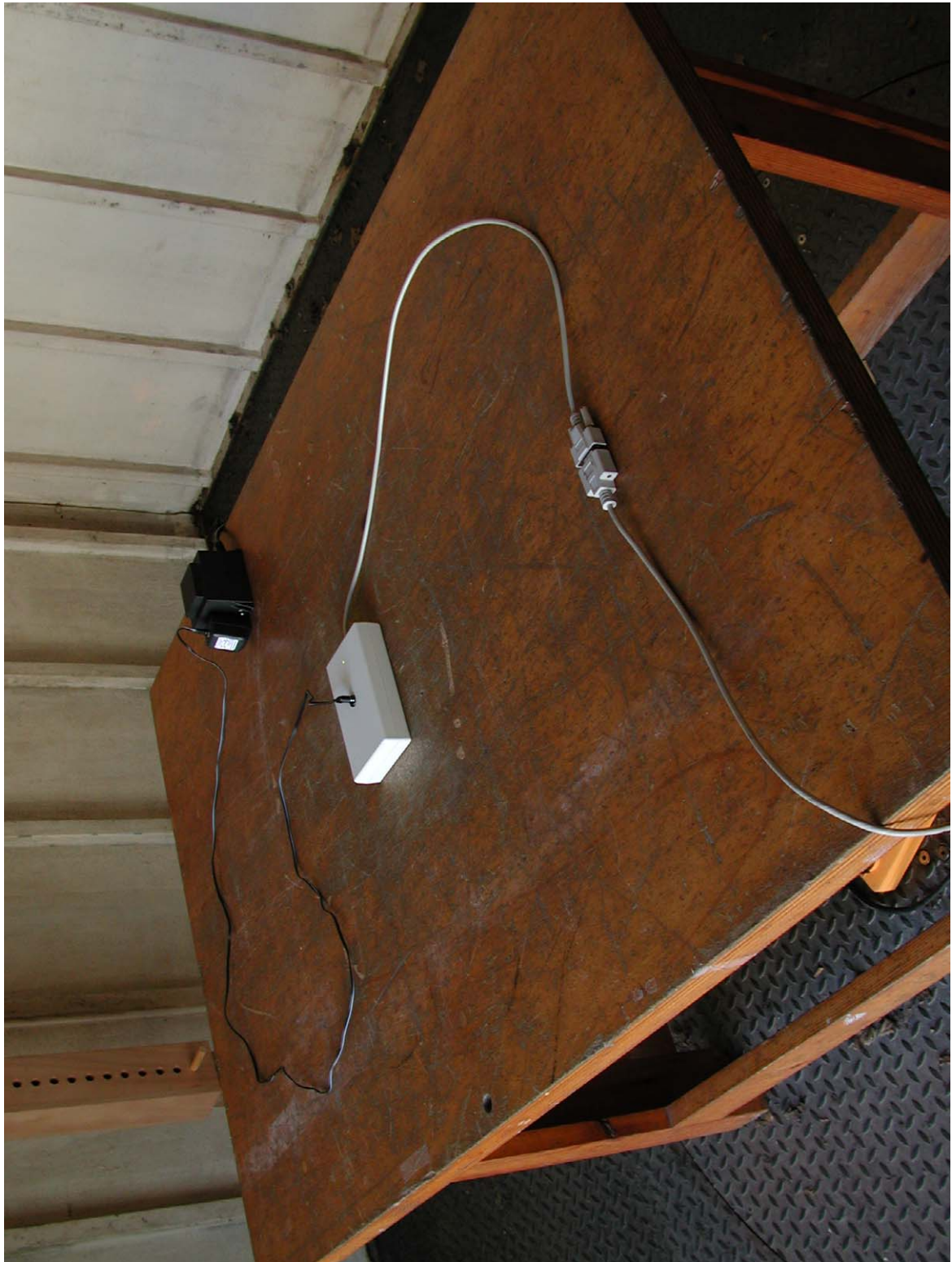
Photograph 9: Test setup radiated emissions < 1 GHz (server on test table)
