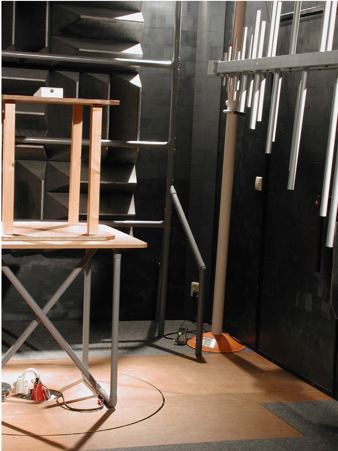
Photograph 4: Test setup exploratory radiated emissions <1 GHz (scoring device)
