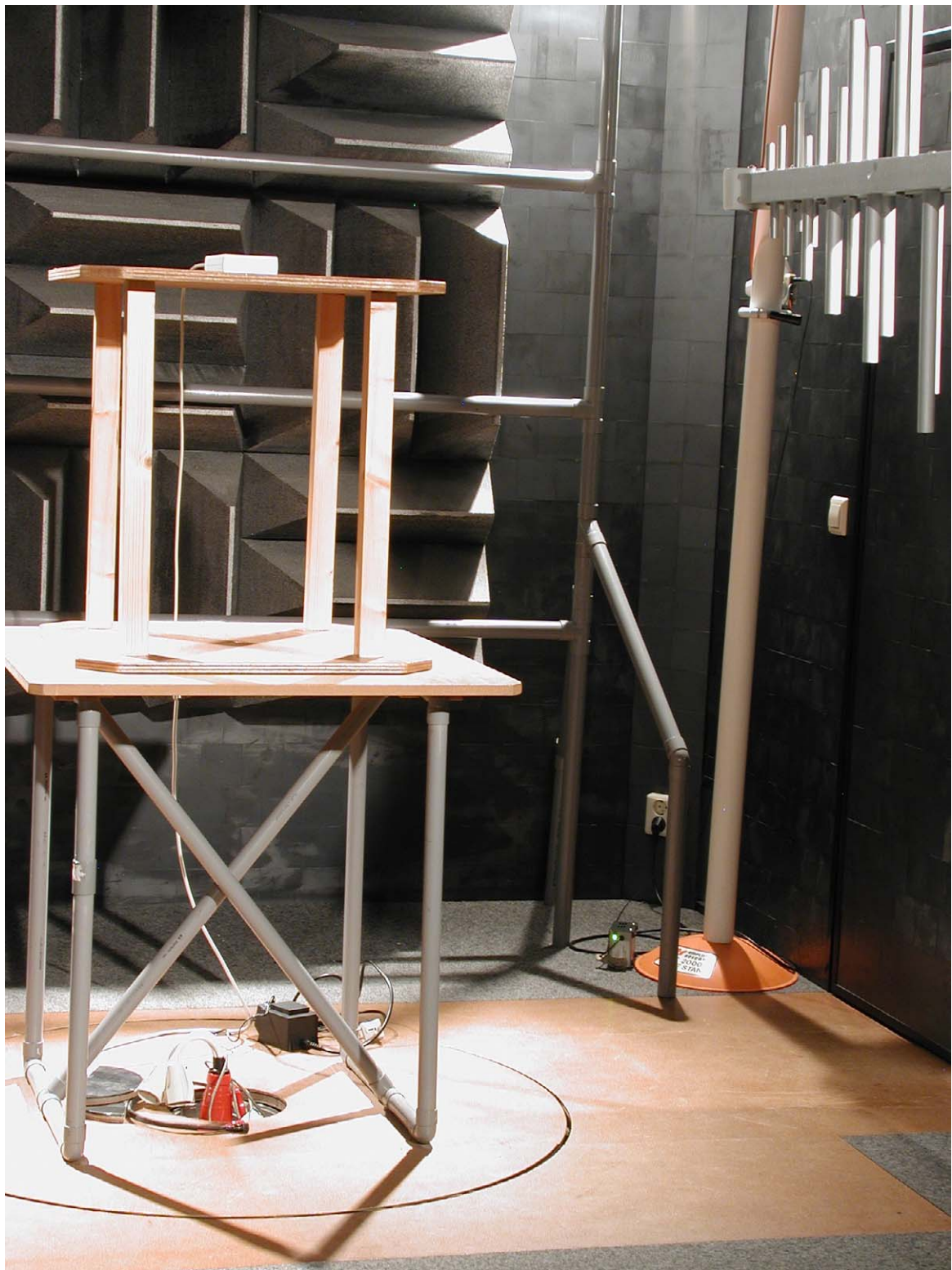
Photograph 5: Test setup exploratory radiated emissions <1 GHz (server)
