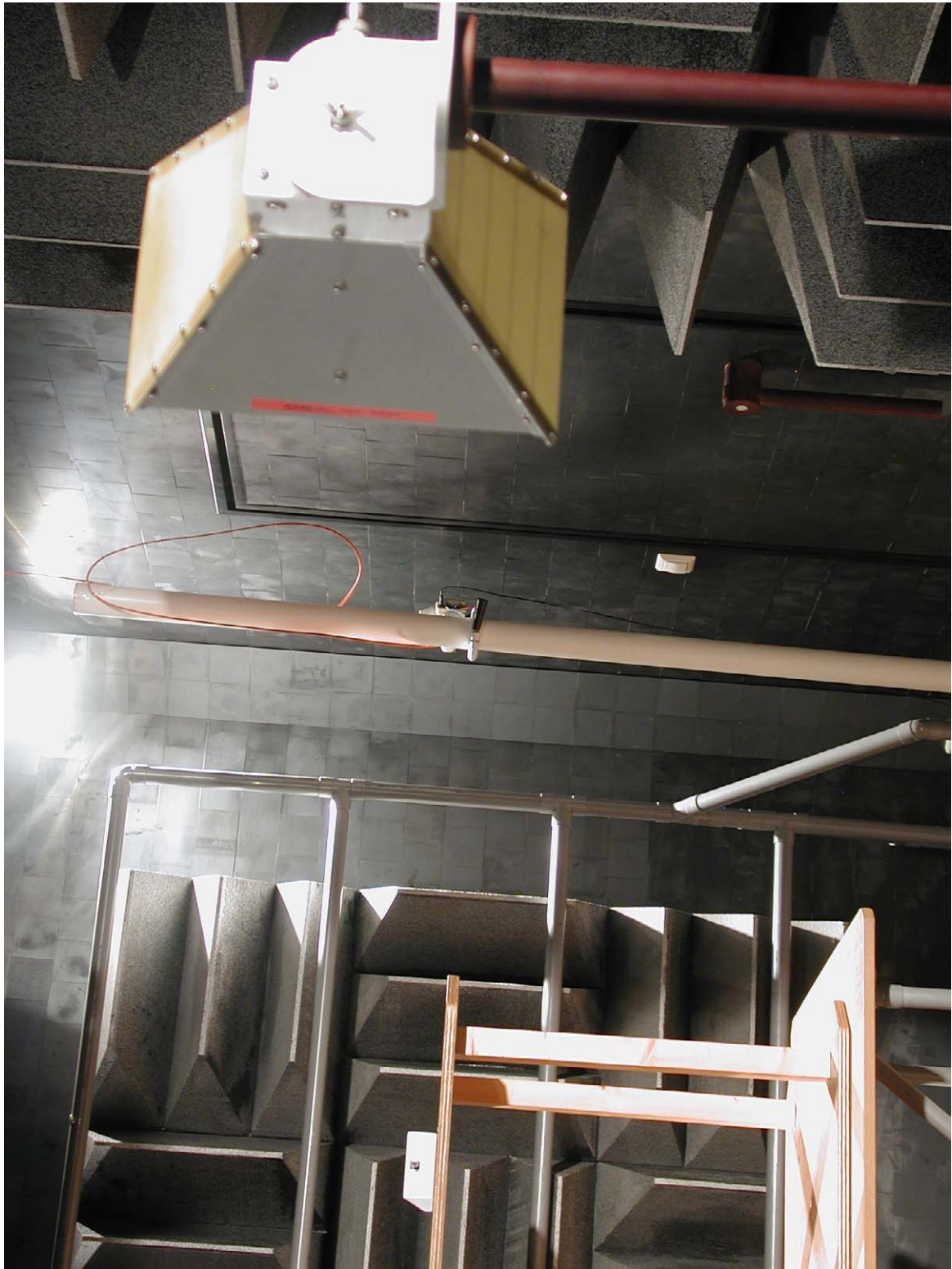
Photograph 10: Test setup radiated emissions > 1 GHz (scoring device)
