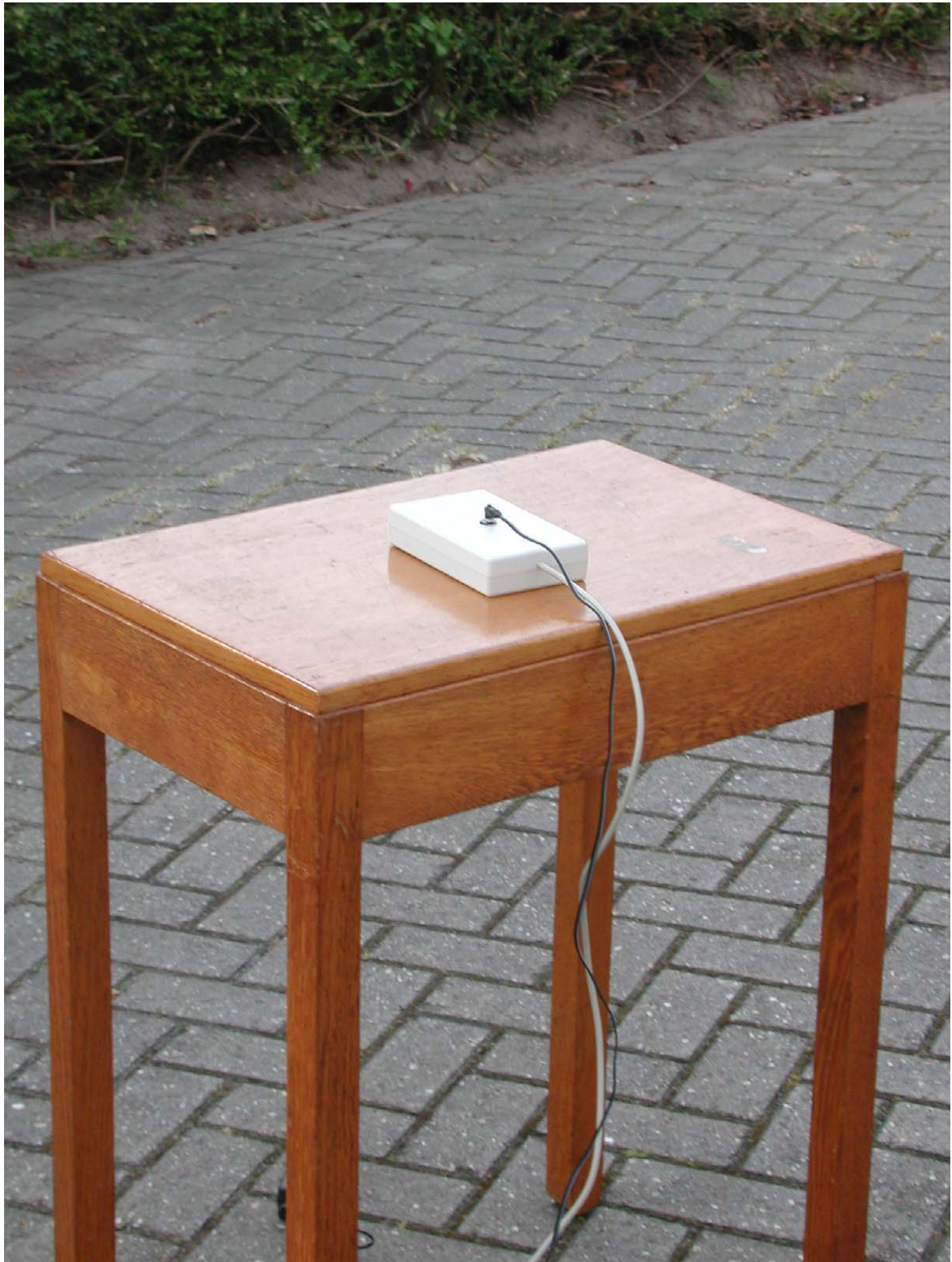
Photograph 2: Test setup radiated emissions <30 MHz (server)
