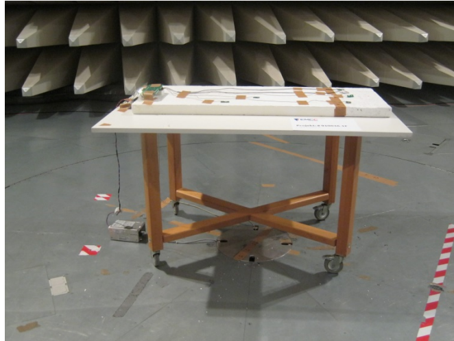
Photograph A1-1: Setup of EUT M21 with all antennas connected
