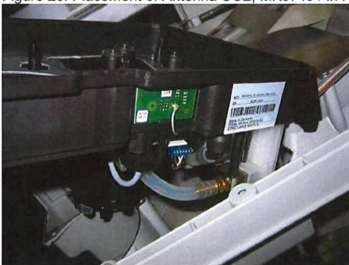
Figure 27: Placement of Antenna Flow In, MK07486, in Perseus A500
