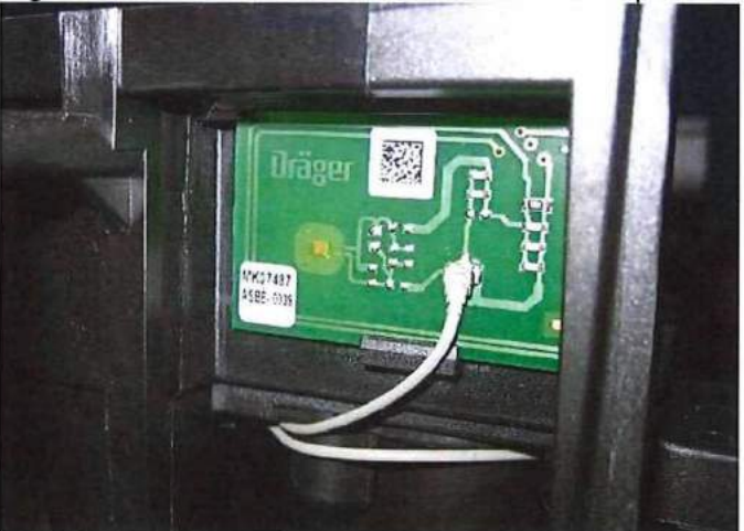
Figure 44: Placement of Antenna Flow Exp 8609931
