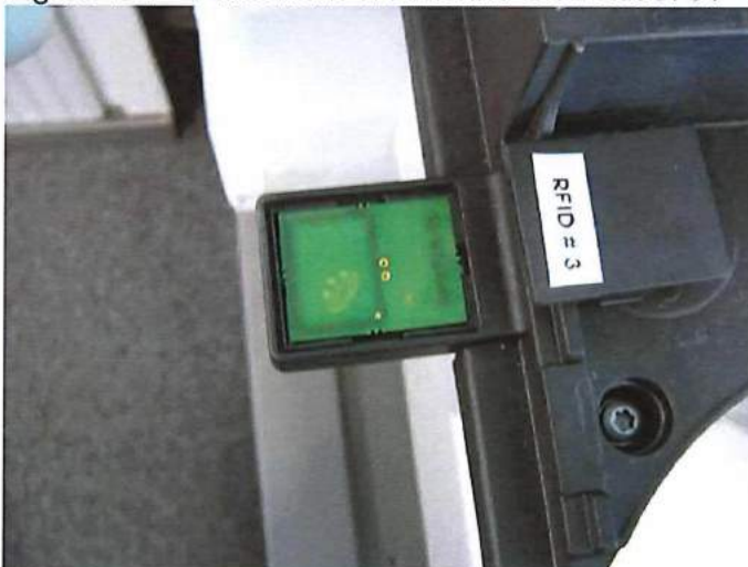
Figure 41: Placement of Antenna Breath Insp 8609741
