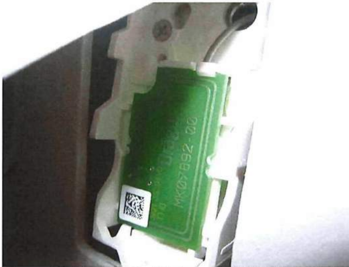
Figure 25: Placement of Antenna WAL, MK07891 in Perseus A500
