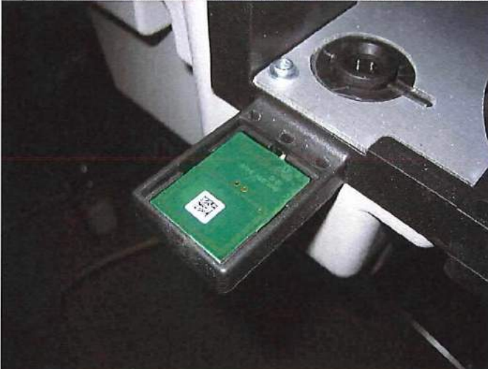
Figure 29: Placement of Antenna Breath In, MK07476 in Perseus A500
