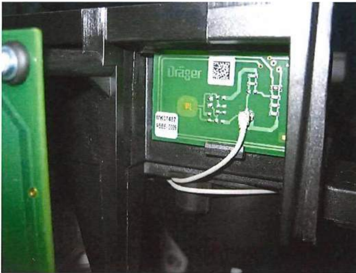
Figure 28: Placement of Antenna Flow Ex, MK07487, in Perseus A500
