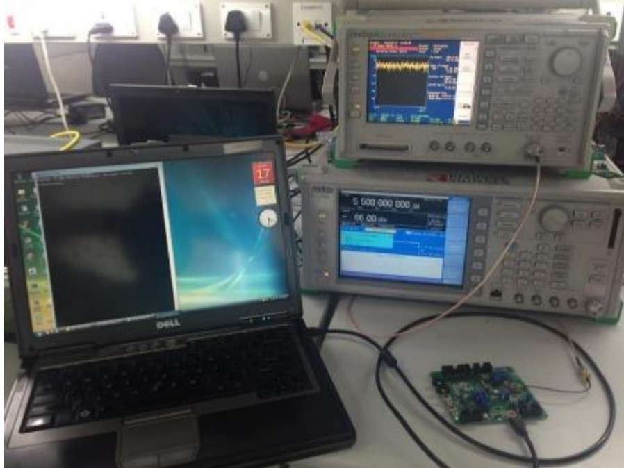
Linux Based RF Evaluation Setup With USB Interface
