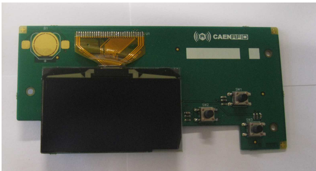
Figure 6: Display Board – Top side
