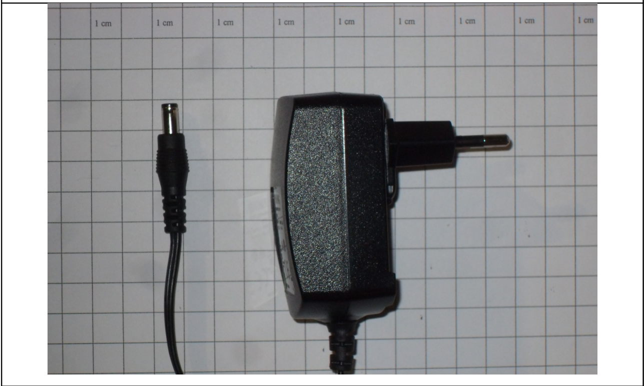
Fig. 1.2 Equipment Photo: Power Supply
