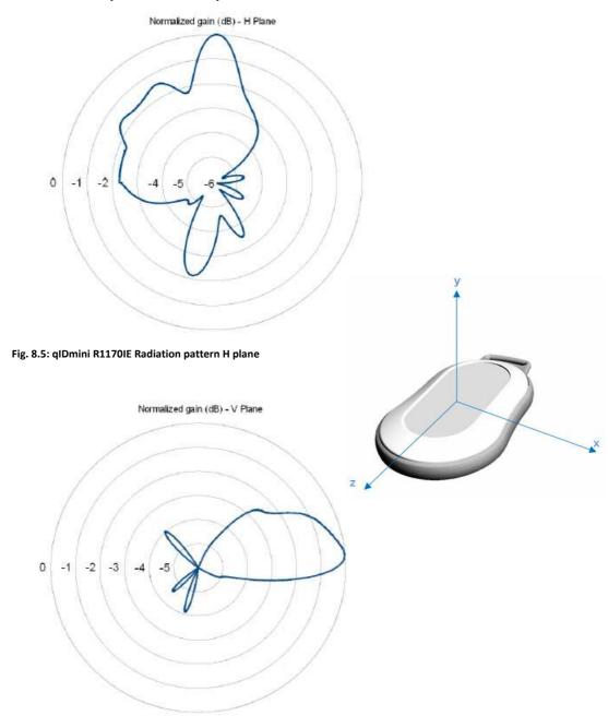
Fig. 8.6: qIDmini R1170IE Radiation pattern V plane
