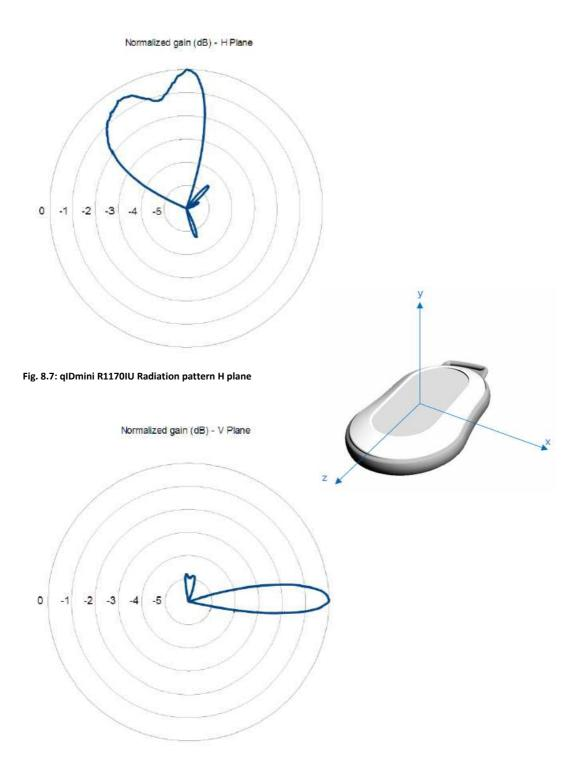
Fig. 8.8: qIDmini R1170IU Radiation pattern V plane
