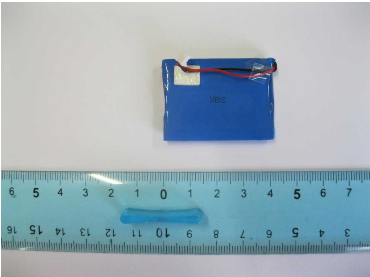
Fig. 14: Li-Pol Battery Bottom View
