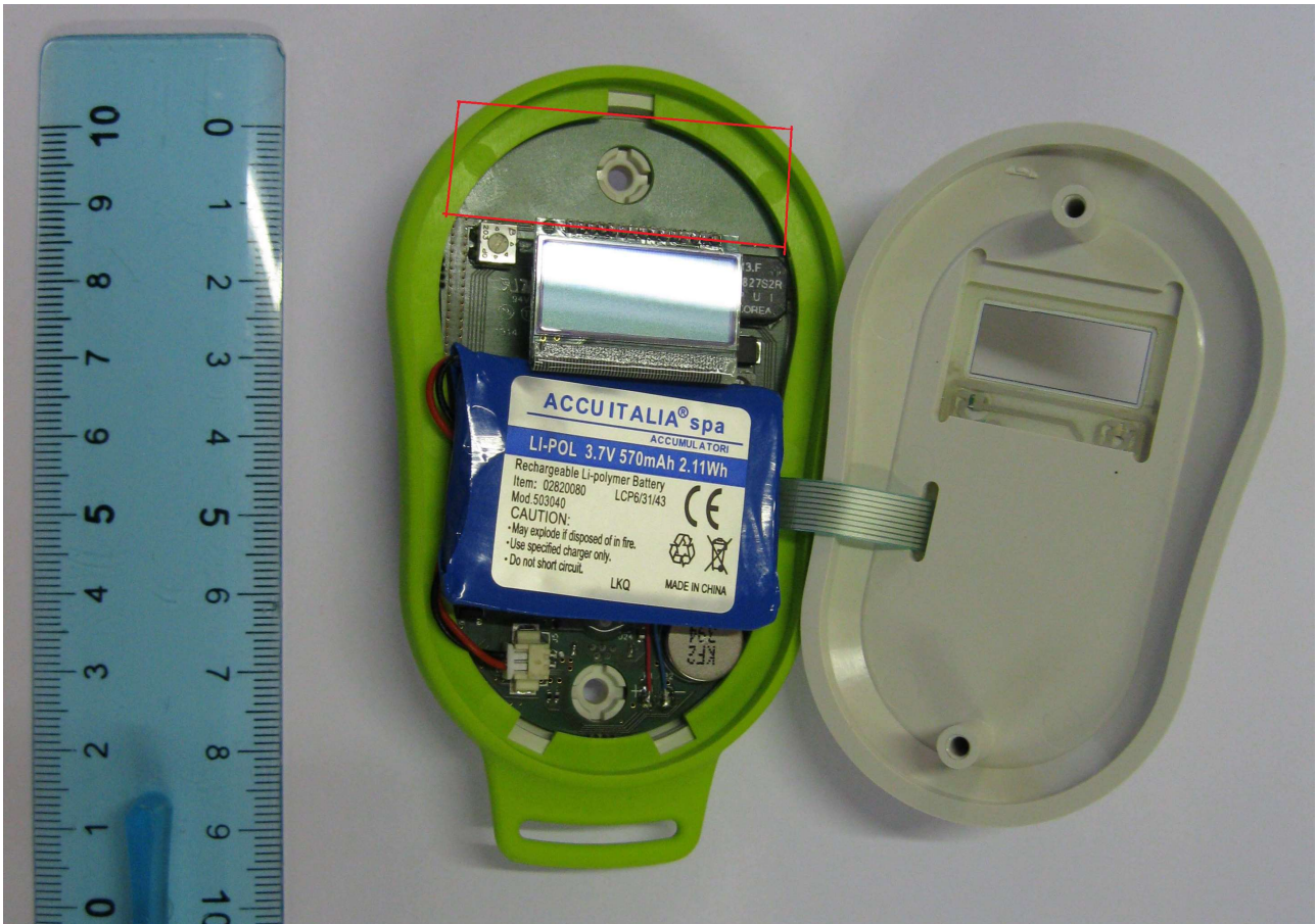
Fig. 4: Antenna location, internal view from top side (antenna trace is on bottom side)
