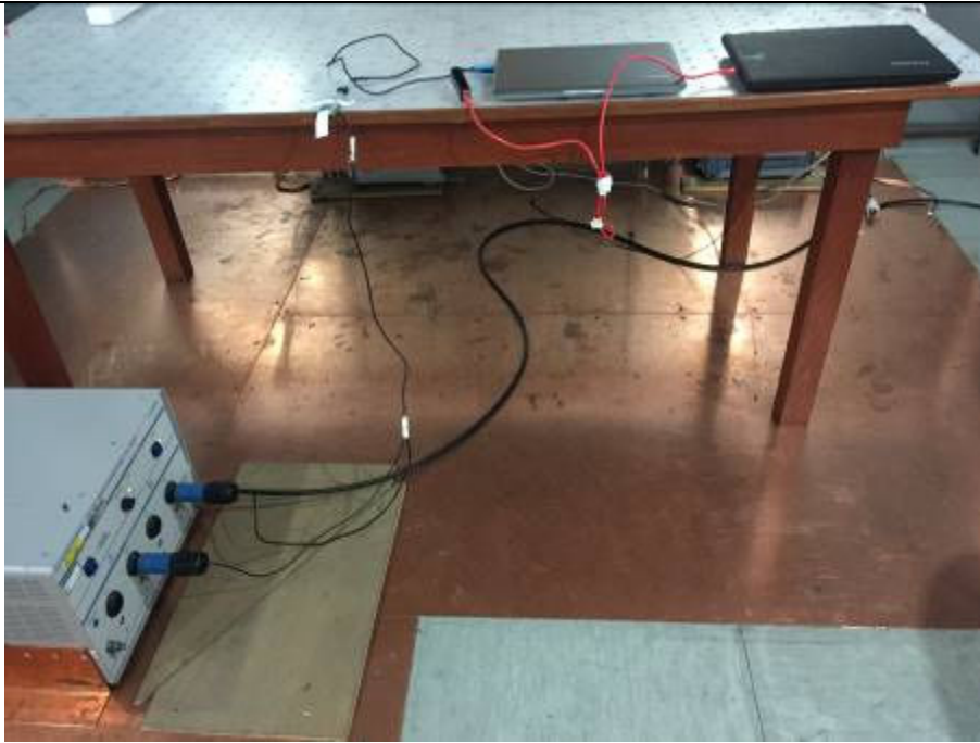
Conducted Emissions Test Setup (with charger)
