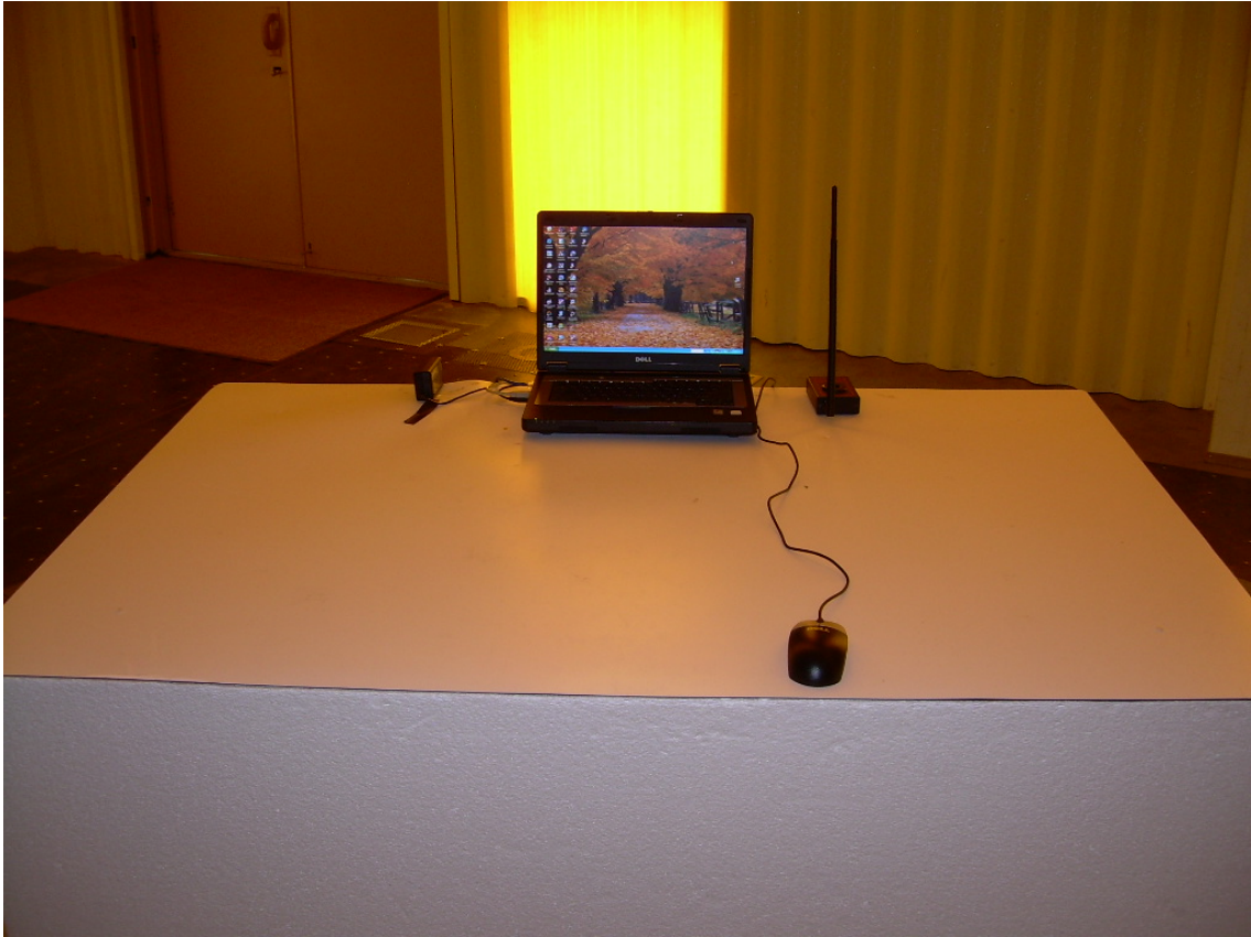
Front View Radiated Spurious Worst Case Configuration - DTENV-H
