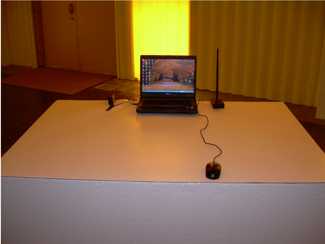
Photograph 1 - Front View Radiated Spurious Worst Case Configuration - DTENV-H
