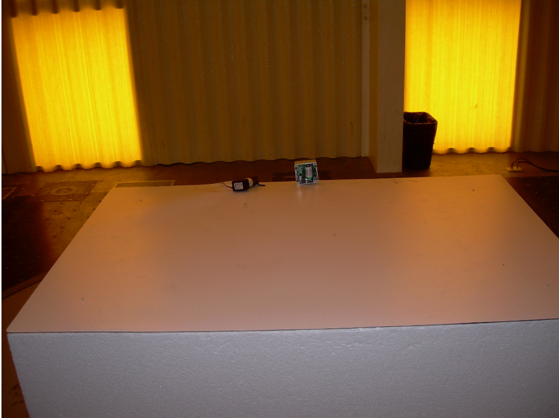
Photograph 3 - Front View Radiated Spurious Worst-Case Configuration - DTENV-R
