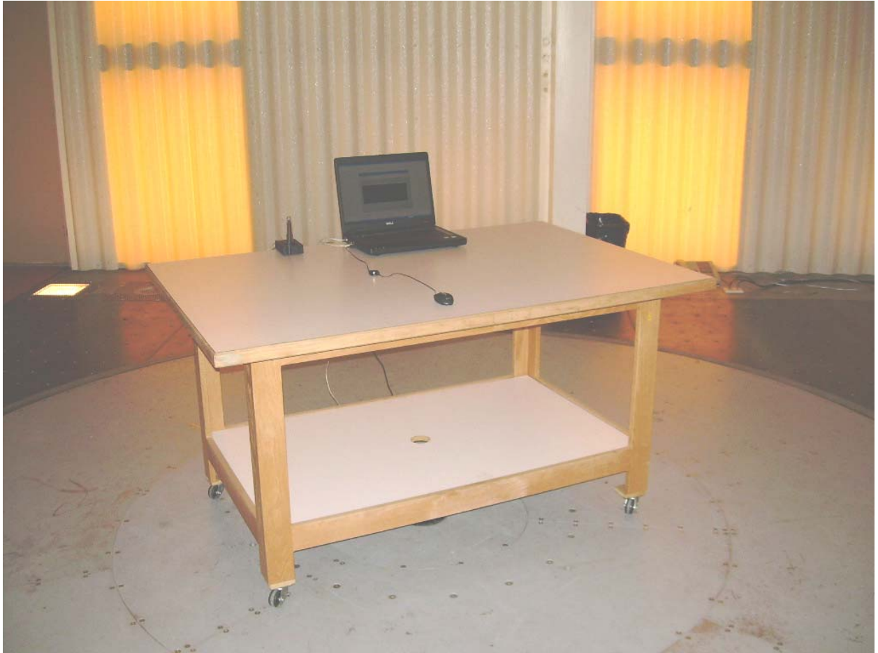
Front View Radiated Disturbance Worst Case Configuration
