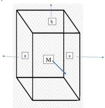
Evaluation is from the full impact of one of the 5 GHz antenna pairs from the front main beam M in addition to the side lobe impact of the antenna pairs from adjacent sides a, b and c.
